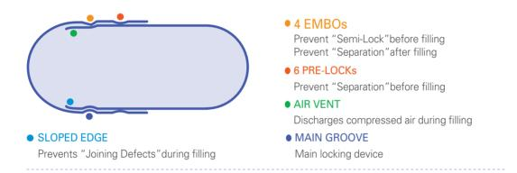
By embossing four dimples on the main locking groove of the cap, the exclusive EMBO CAPS® is designed to offer distinct advantages.
